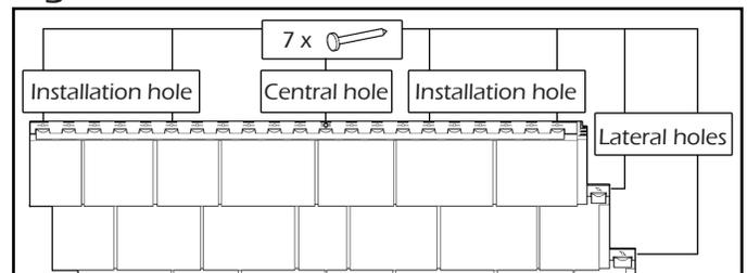
4-Install the following panel by hooking it into the starter strip and sliding it to the left overlapping the previous panel. Make sure to properly engaged the lateral hooks and spaced equally the panels according to the outdoor temperature during the installation. See temperature marks on panels (Figure D).
