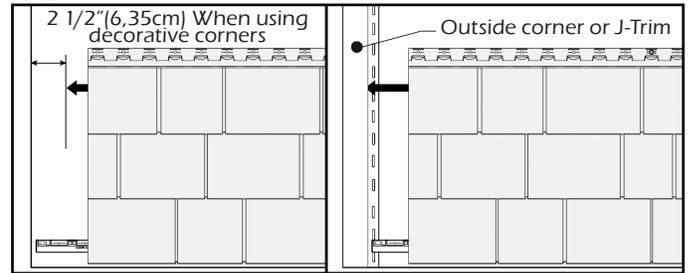
3-On each panel, hammer a nail into the center hole of the panel, this will ensure even movement of panel in both directions during expansion/contraction. Also hammer a nail into the last hole on both ends, plus 2 other nails into nailing channel and a nail in each lateral holes (Figure C). Each full length panel should be secured with a minimum of 7 nails. If the panel is installed on a furring wall, a furring strip is required behind each nail.\*
