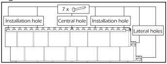
4-Install the following panel by hooking it into the starter strip and sliding it to the left overlapping the previous panel. Make sure to properly engaged the lateral hooks and spaced equally the panels according to the outdoor temperature during the installation. See temperature marks on panels (Figure D). Installation:
