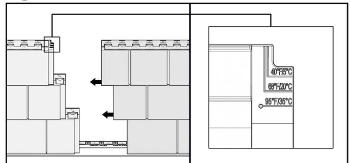
5-Begin the second row by cutting the first panel with approximately 16"(40,64cm) increment from the cutting line of the first row. Hooking the lower panel section with the top hooks of the last installed row. To eliminate stacking seams, alternate the cut positions for the following rows. (Figure E)
