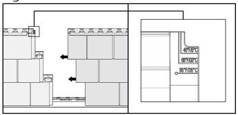
5-Begin the second row by cutting the first panel with approximately 16"(40,64cm) increment from the cutting line of the first row. Hooking the lower panel section with the top hooks of the last installed row. To eliminate stacking seams, alternate the cut positions for the following rows. (Figure E)
