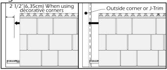
3-On each panel, hammer a nail into the center hole of the panel, this will ensure even movement of panel in both directions during expansion/contraction. Also hammer a nail into the last hole on both ends, plus 2 other nails into nailing channel and a nail in each lateral holes (Figure C). Each full length panel should be secured with a minimum of 7 nails. If the panel is installed on a furring wall, a furring strip is required behind each nail.\*
